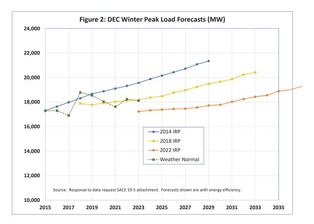
20. The 2022 forecasts appear lower than the trends in the recent weather-normalized peaks. However, the weather-normalized peaks may be somewhat overstated. The weather-normalized values average 688 MW higher than the actual peaks for summer and 484 MW higher than the actual peaks for winter over the 2011 to 2022 period.<sup>16</sup> Taking this into account, the 2022 forecasts were reasonably consistent with the past trends.
