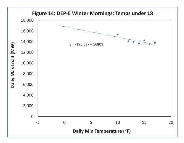
59. For DEP-East, focusing the analysis on temperatures below 18 degrees lowers the estimate from the 248.28 MW/degree value noted above to 195.58, as shown in Figure 14.
