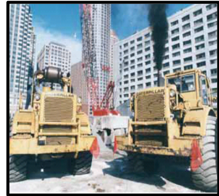
Construction equipment WITHOUT a filter emits high levels of black carbon. (on right)
