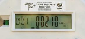
Type FOCUS AXR-SD FORM 2S CL200 240V 3W 60Hz TA=30 Kh 7.2
